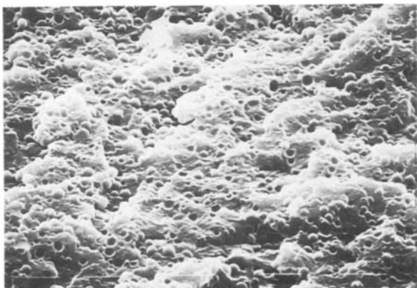
Figure 9 SEM micrograph of Izod fracture surface of 90/10 PA6/Elvax 220 blend (1900 ×) (central region).
