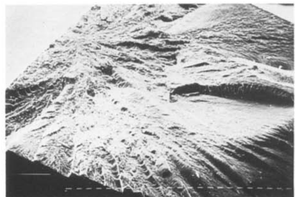
Figure 16 SEM micrograph of Izod fracture surface of 80/20 PA6/Elvax 40 blend (30 ×).
