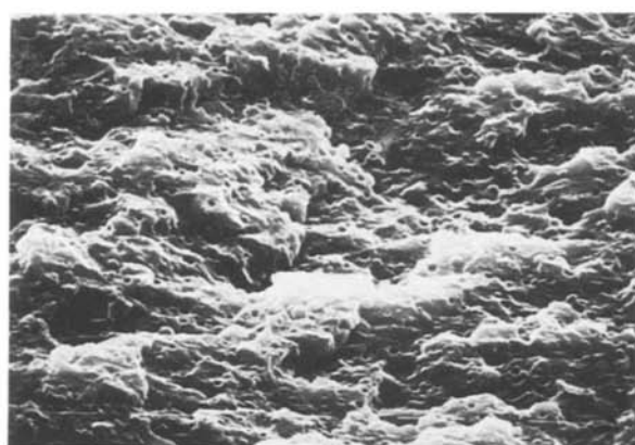
Figure 8 SEM micrograph of Izod fracture surface of 95/5 PA6/Elvax 220 blend (1900 ×) (central region).
