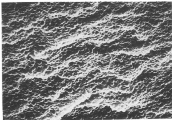
Figure 7 SEM micrograph of Izod fracture surface of 80/20 PA6/Elvax 220 blend (1900 ×) (central region).
